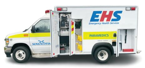
While the ambulance module is remounted, it is repaired, painted, and the latest technologies and layouts can be retrofitted. This type of remount allows for a lower cost with similar functionality to a new vehicle.
